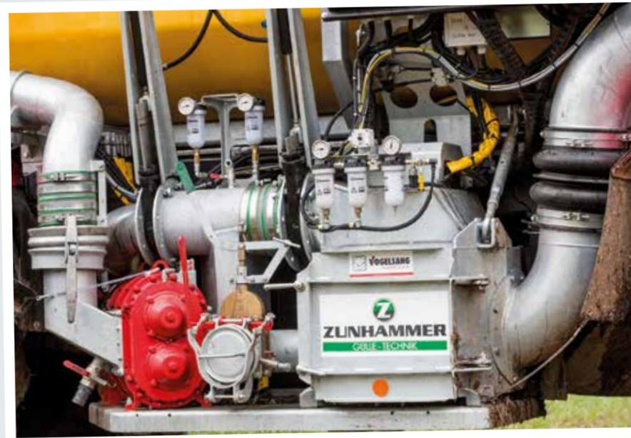
During filling, up to 9000 litres per minute can be transferred with the Vogelsang rotary pump. The red unit positioned next to the pump is the Rotocut, which has automatic cutting control to maintain pressure and automatic reversing to avoid blockages.
