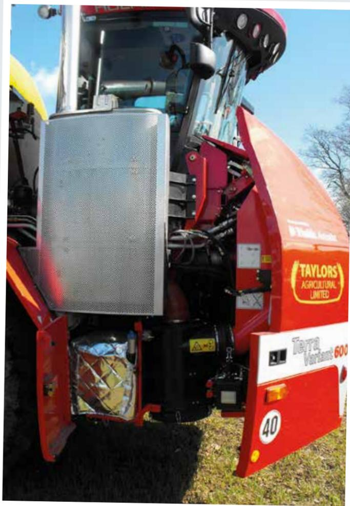
The 598hp engine can be accessed via wide opening panels, and the cab can be tilted forward for easy maintenance.
