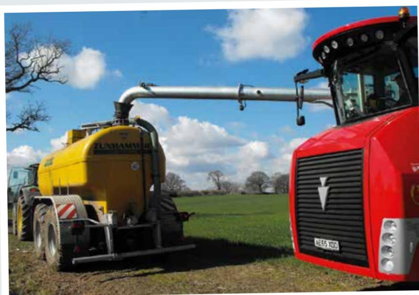
The 10" diameter, 5.7m suction pipe pivots up to 17° and can operate at any point for filling over hedgerows and ditches. This means that operation can continue and efficiency can be maintained even if the tankers are not able to access the field.
