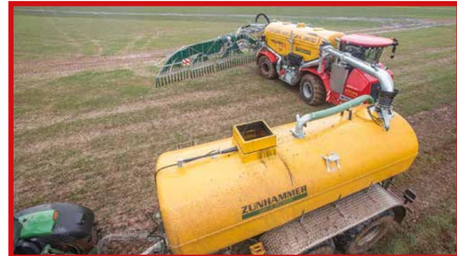
*High product flow during filling means that the 18m<sup>3</sup> tankers can be emptied in just over two minutes, meaning the Taylors can maintain a level of efficiency despite their distance from the plant.*
