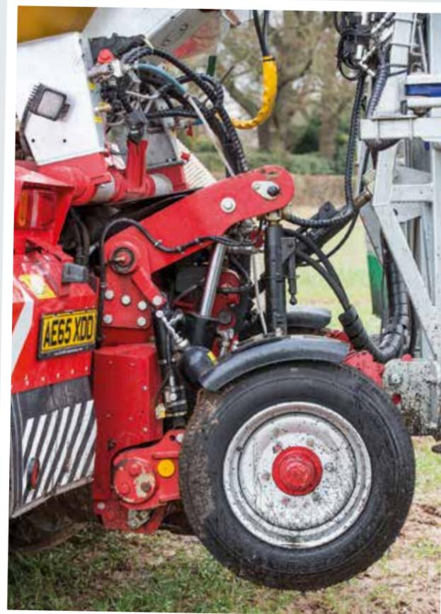
The dribble bar is mounted on a fully hydraulic, pivoting three-point mount to keep the unit in a straight line at all times, even when operating in crab steer mode. The linkage also means that cultivators specified to apply slurry can be operated behind the tanker for product integration.
