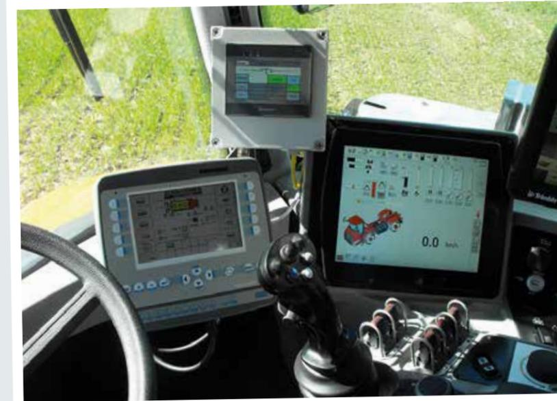
The Holmer specified by the Taylors has four terminals fitted, one for each aspect of the unit and a Trimble FmX screen for guidance. Most functions are controlled either through the Holmer terminal or the multi-function joystick, with a minimum of switches and dials at the side of the operator.
